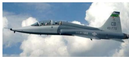
Northrop T-38 Talon Max Speed – 814 kts/ 1.23 Mach Cruise/Pattern airspeed – 300 kts Final airspeed – 160 kts
